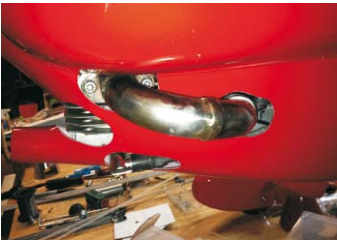
The final cut out in the firewall to allow the carby to sit back further. (Some Heavy Model Inspectors are uncomfortable with this due the to possibility of an engine backfire and fumes inside the fuselage. Ed)
