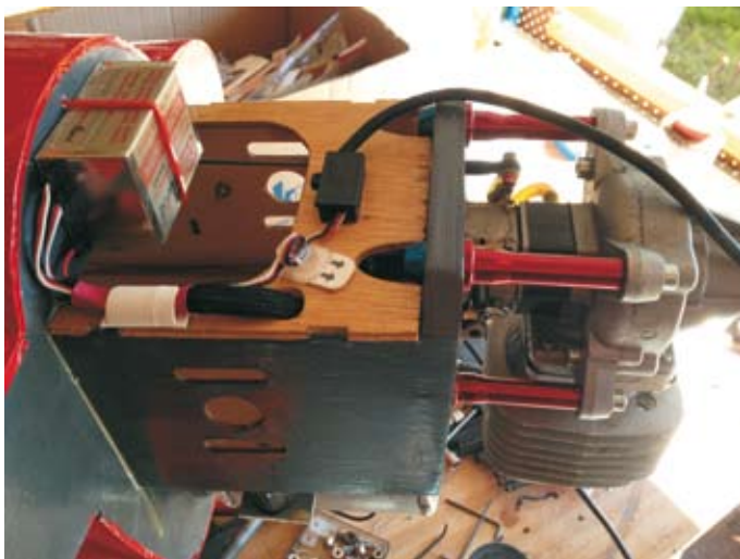
Above left, new engine box top plate mounted
