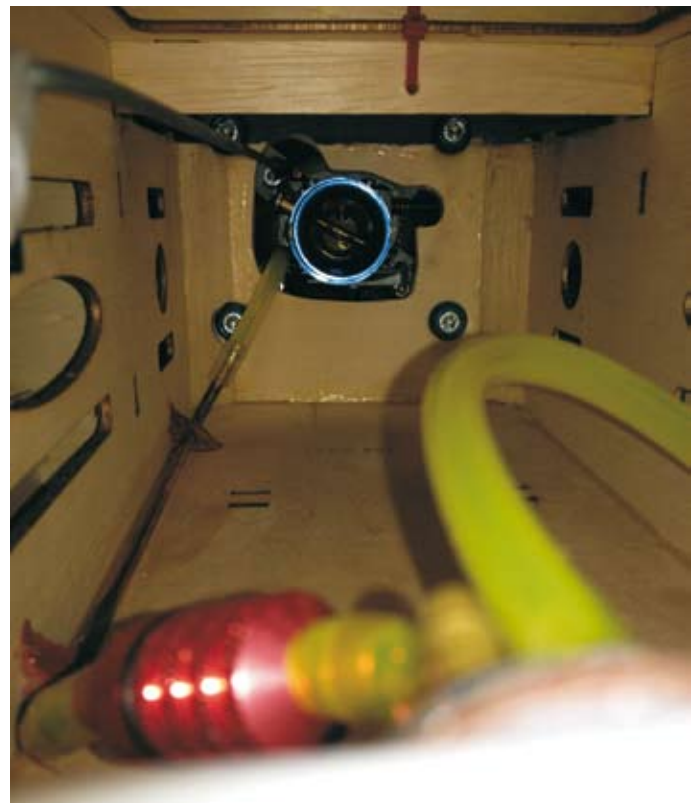
The final cut out in the firewall to allow the carby to sit back further. (Some Heavy Model Inspectors are uncomfortable with this due the to possibility of an engine backfire and fumes inside the fuselage. Ed)
