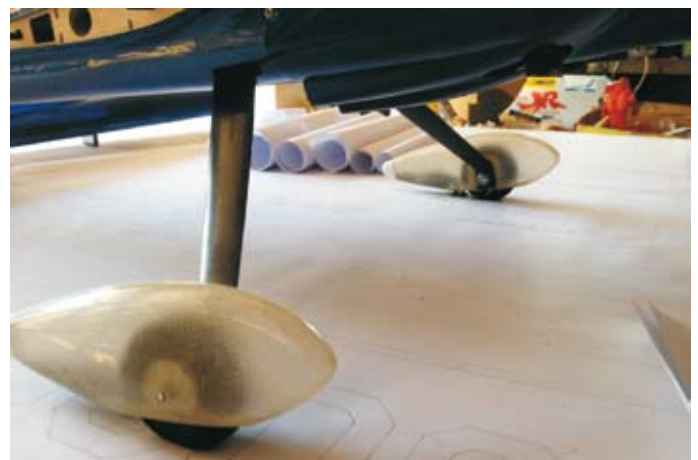
Syssa 30 cc petrol and APC 15x14, Bolly carbon undercarriage
