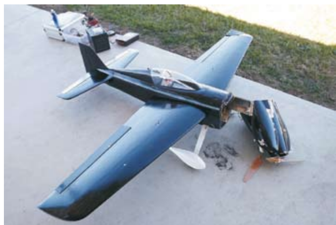
Jay Everitt's Nemesis. The donk flew out in flight rounding Pylon 1. Problem was caused by excessive vibration after the spinner came off and damaged the propeller. Model floated down and survived relatively intact
