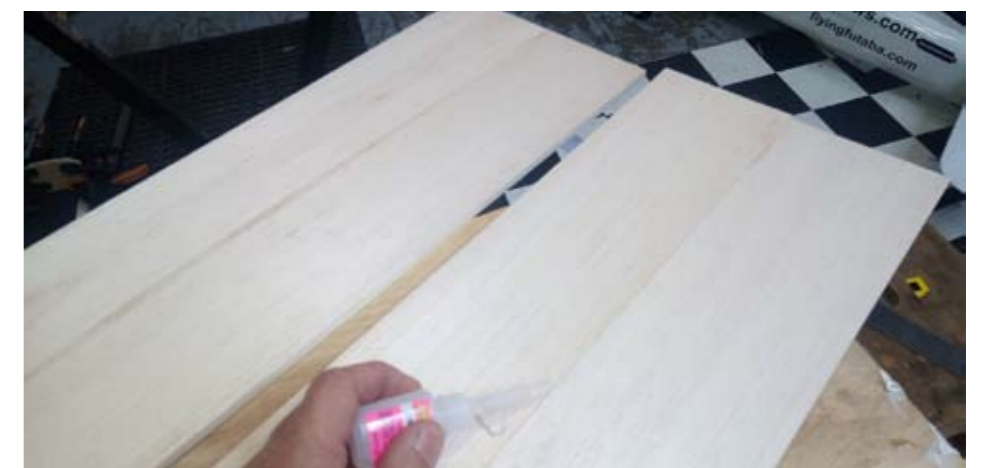
Splicing fuselage sides
