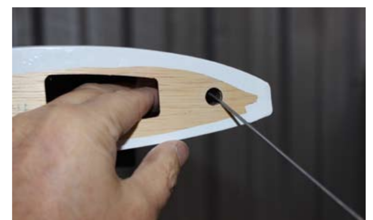
Loose blind nut fix B
