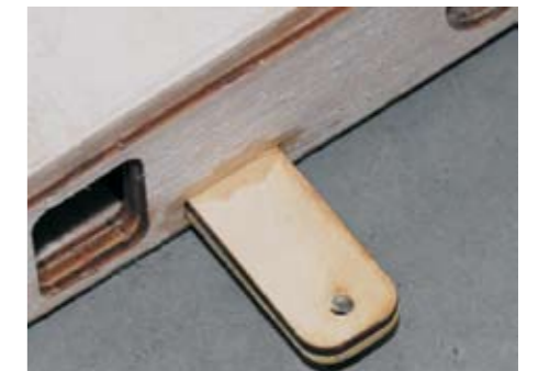
Wicking in thin cyano is the easiest way to prevent this coming loose
