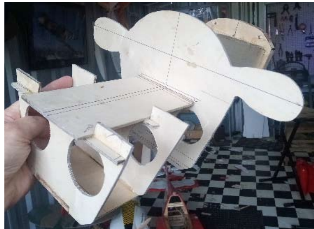
Engine box with undercarriage and tank mounts
