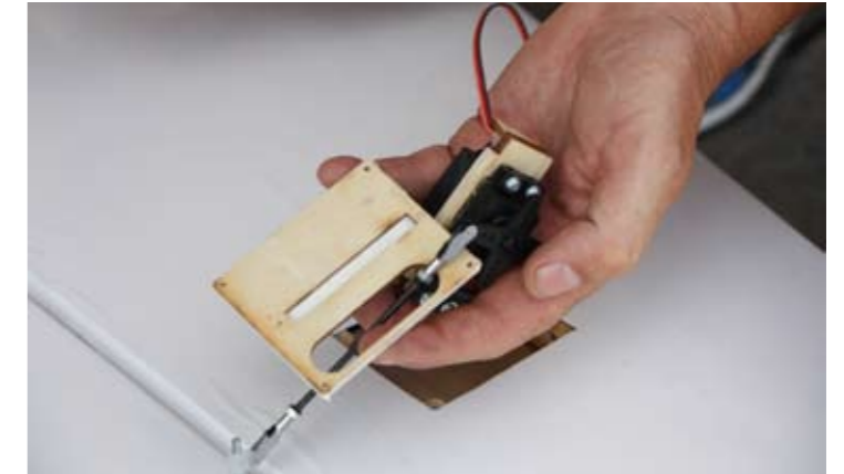
Wicking in thin cyano is the easiest way to prevent this coming loose
