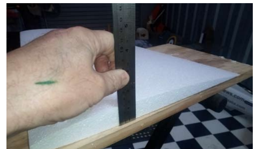
25mm thick MH30 aerofoil for 2mm balsa skins
