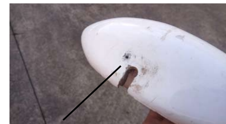
Bolt drilled through undercart leg acts as anti rotation pin
