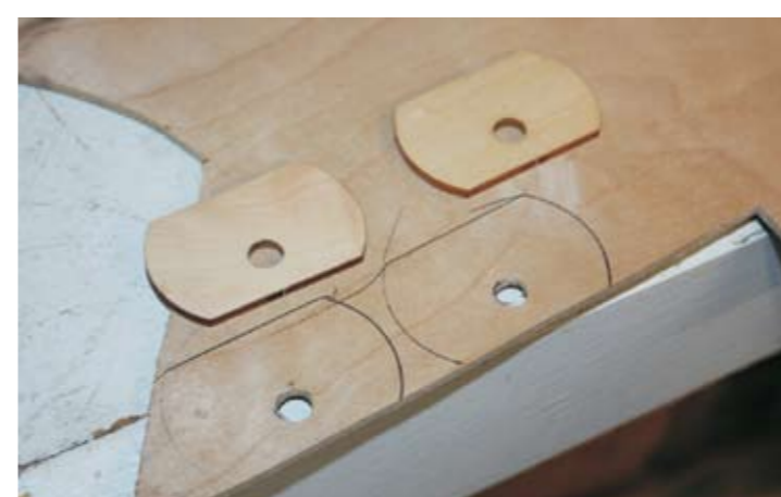
Hard ply wheel spat flanges
