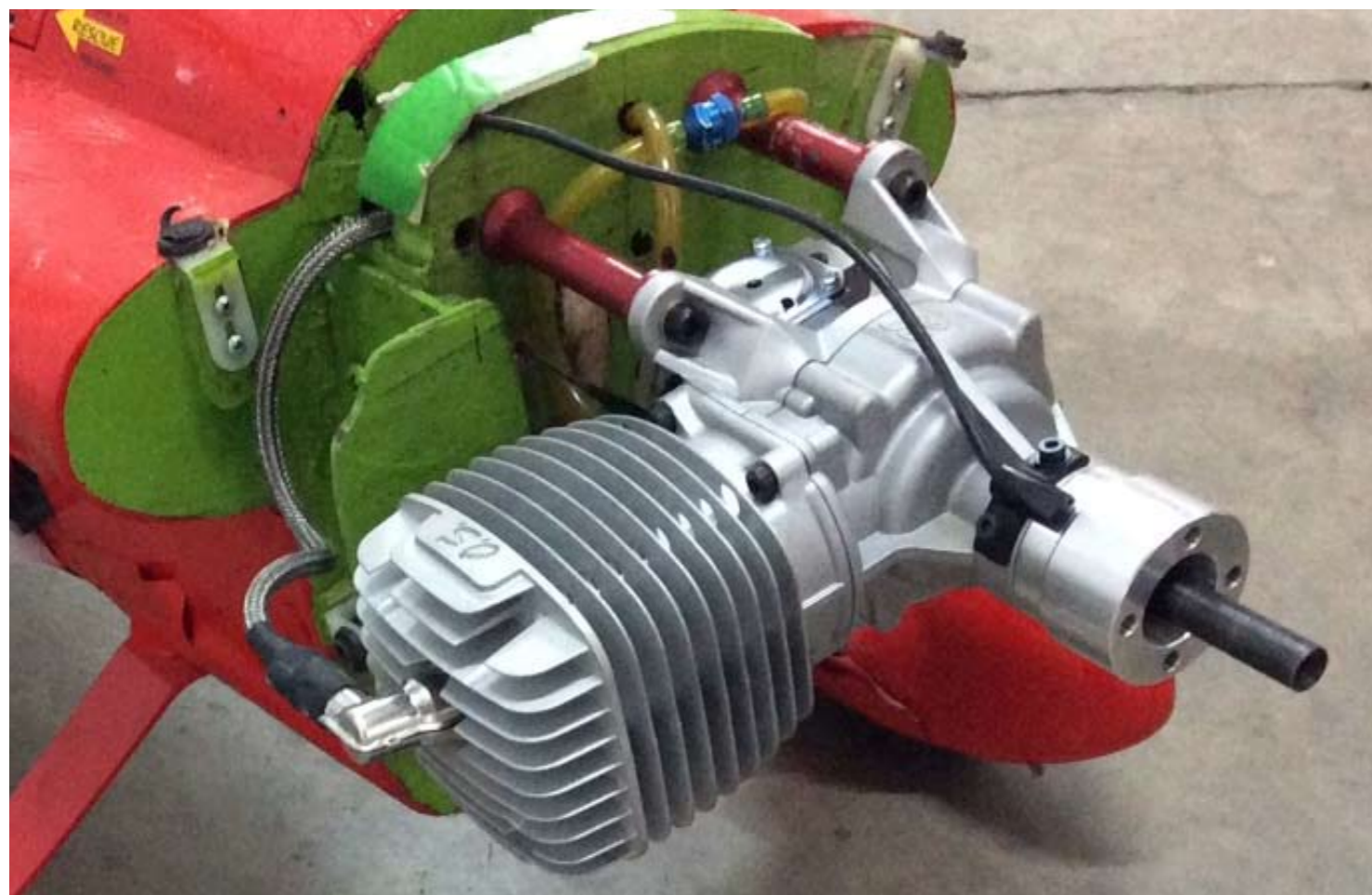
Fire-wall replaced with two pieces of 6.5mm aircraft or marine grade plywood with 1.5 mm ply doubler each side of the engine box
