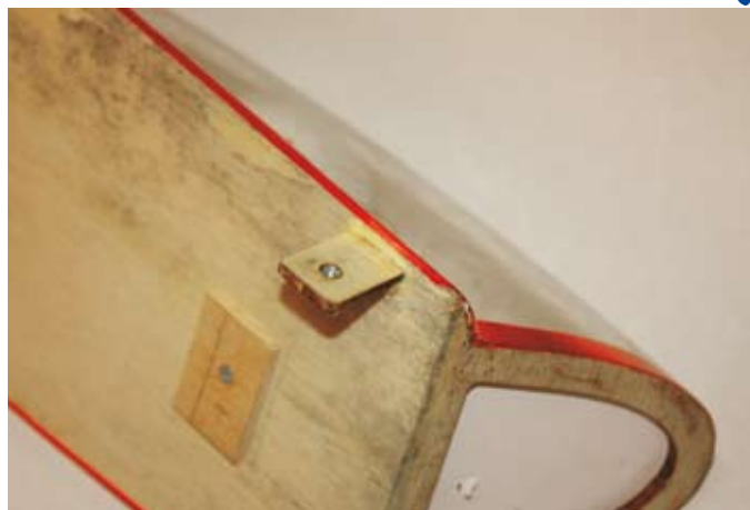
Insufficient tension can be applied to secure canopy bolts. Mount flexes when bolts are tightened.
