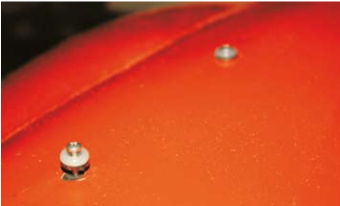
Soft ply plate compressed and axle nut fell off
