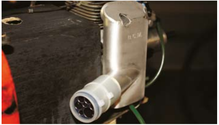
Side mount Bisson muffer for OS GT 55 in the Nemesis. DL engines exhaust button reduced the noise level 3db
