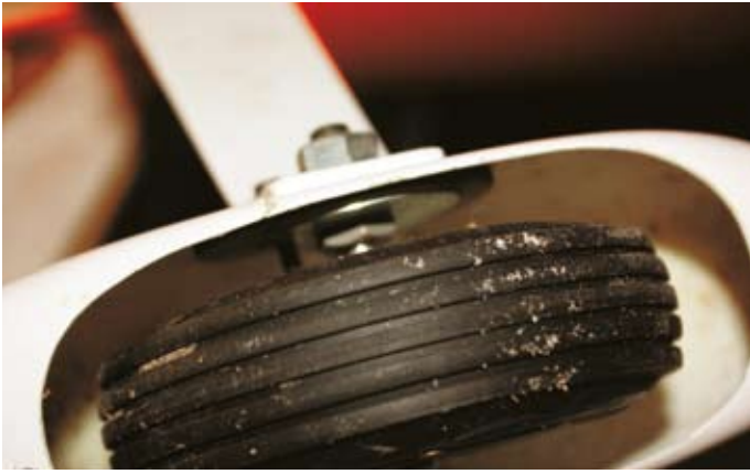
Soft ply plate compressed and axle nut fell off
